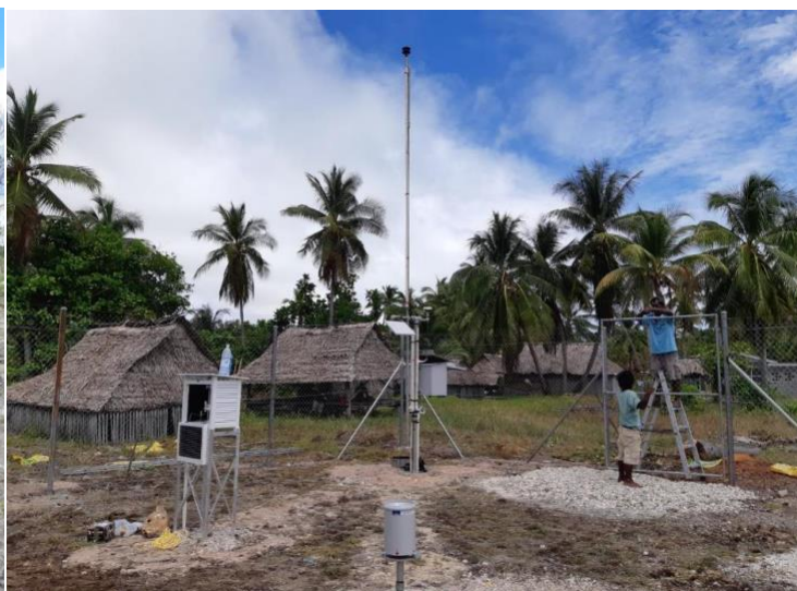
Figure 4 Abemama AWS – tipping bucket rain gauge in foreground, Fairmount screen on left, and mast behind.
