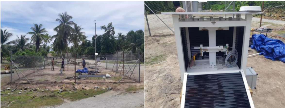
Figure 1a. AWS at Maiana and 1b. Maiana AWS – 1b) Screen with air temperature and humidity sensor, Licor solar radiation on top right
