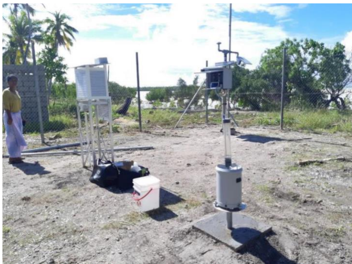
Figure 3 Nonouti AWS – tipping bucket rain gauge
